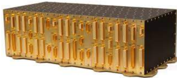
Figure 4.3: Power conditioning and distribution unit developed by Terma Space for the Galileo mission (Terma Space, 2016).
