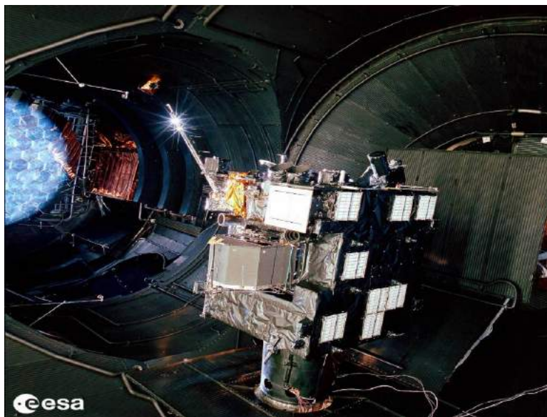
Figure C.3: The white rectangles on the Rosetta spacecraft shown above are the louvres which are similar to the ones planned for OCEANUS.
