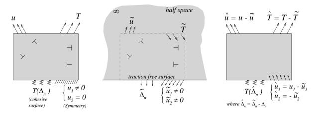
**Figure 3**: Decomposition of the problem into the problem of interacting dislocation in the homogeneous free-traction half space ( $^{\sim}$  fields) and the complementary problem of the elastic body without dislocations ( $^{\wedge}$  fields).
