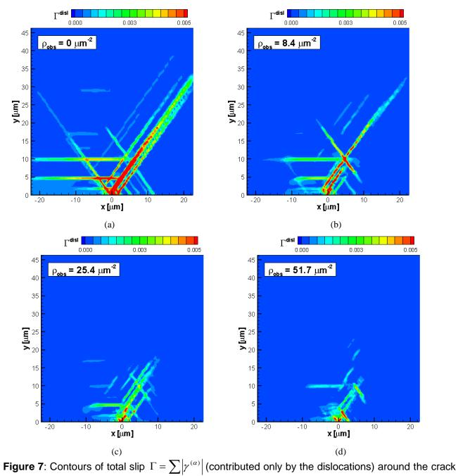
**Figure 7**: Contours of total slip  $\Gamma = \sum |\gamma^{(\alpha)}|$  (contributed only by the dislocations) around the crack tip at  $K_l/K_0 = 0.08$ . (a)  $\rho_{obs} = 0 \ \mu m^{-2}$ , (b)  $\rho_{obs} = 8.4 \ \mu m^{-2}$  (c)  $\rho_{obs} = 25.4 \ \mu m^{-2}$  (d)  $\rho_{obs} = 51.7 \ \mu m^{-2}$  (e)  $\rho_{obs} = 103.4 \ \mu m^{-2}$  (f) Elastic solution.
