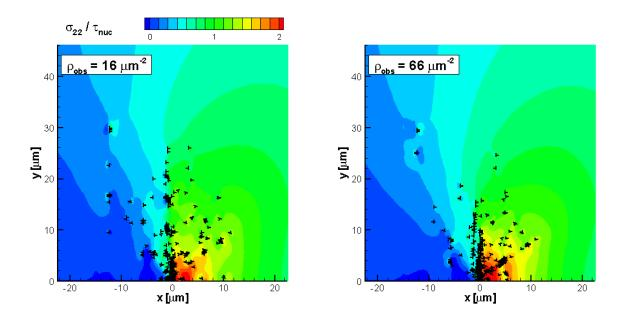
**Figure 14:** Normalized opening stress  $\sigma_{22}/\sigma_{max}$  and dislocation distribution at  $K_I/K_0 = 0.08$  for the bcc-like orientation and two different obstacle densities: (a)  $\rho_{obs} = 16 \ \mu m^{-2}$ , (b)  $\rho_{obs} = 66 \ \mu m^{-2}$ .
