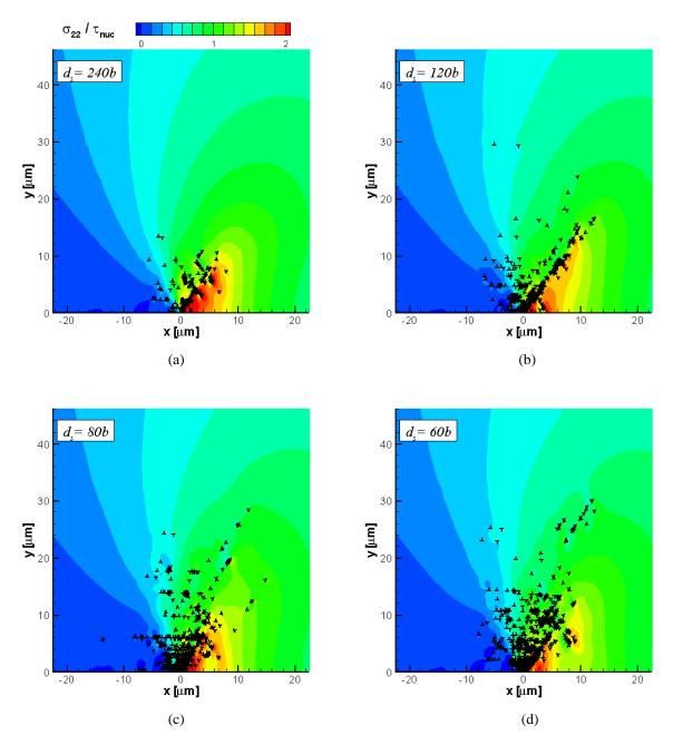
**Figure 9:** Normalized opening stress  $\sigma_{22}/\sigma_{max}$  and dislocation distribution at  $K_l/K_0 = 0.08$  for different slip planes spacing: (a)  $d_s = 240$  b, (b)  $d_s = 120$  b, (c)  $d_s = 80$  b, and (d)  $d_s = 60$  b.
