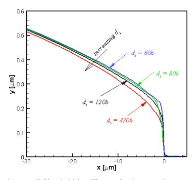
**Figure 13**: Crack shape at  $K_1/K_0 = 0$ . 08 for different slip plane spacing.
