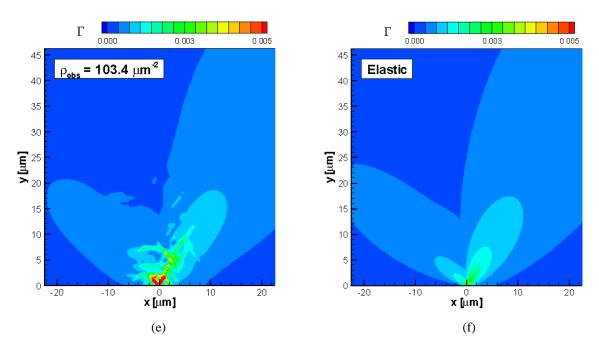
Figure 6 (cont.): Contours of total slip  $\Gamma = \sum |\gamma^{(\alpha)}|$  around the crack tip at  $K_I/K_0 = 0.08$ . (a)  $\rho_{obs} = 0$  μ $m^{-2}$ , (b)  $\rho_{obs} = 8.4 \ \mu m^{-2}$  (c)  $\rho_{obs} = 25.4 \ \mu m^{-2}$  (d)  $\rho_{obs} = 51.7 \ \mu m^{-2}$  (e)  $\rho_{obs} = 103.4 \ \mu m^{-2}$  (f) Elastic solution.
