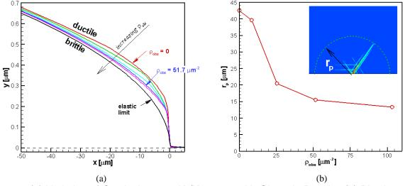
**Figure 8**: (a) Variation of Crack shape at  $K_l/K_0 = 0.08$  with Obstacle Density. (b) Plastic zone size  $(r_p)$  vs obstacle density at  $K_l/K_0 = 0.08$ .
