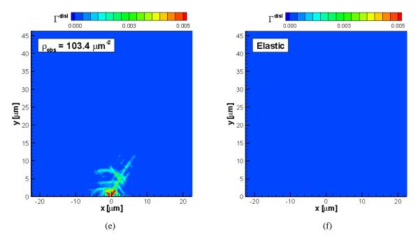
Figure 7(cont.): Contours of total slip  $\Gamma = \sum \left| \gamma^{(\alpha)} \right|$  (contributed only by the dislocations) around the crack tip at  $K_I/K_0 = 0.08$ . (a)  $\rho_{obs} = 0 \ \mu m^{-2}$ , (b)  $\rho_{obs} = 8.4 \ \mu m^{-2}$  (c)  $\rho_{obs} = 25.4 \ \mu m^{-2}$  (d)  $\rho_{obs} = 51.7 \ \mu m^{-2}$  (e)  $\rho_{obs} = 103.4 \ \mu m^{-2}$  (f) Elastic solution.
