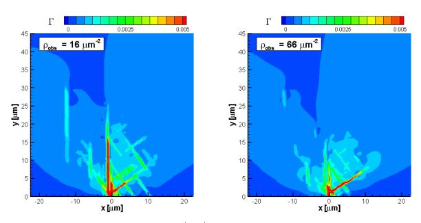
**Figure 15**: Contours of total slip  $\Gamma = \sum \left| \gamma^{(\alpha)} \right|$  around the crack tip at  $K_I/K_0 = 0.08$  for the bcc-like orientation and two different obstacle densities: (a)  $\rho_{obs} = 16 \ \mu m^{-2}$ , (b)  $\rho_{obs} = 66 \ \mu m^{-2}$ .
