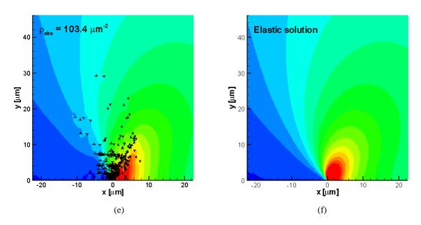
**Figure 4 (cont.)**: Normalized opening stress  $\sigma_{22}/\tau_{nuc}$  and dislocation distribution at  $K_I/K_0 = 0.08$ . (a)  $\rho_{obs} = 0 \ \mu m^2$ , (b)  $\rho_{obs} = 8.4 \ \mu m^2$  (c)  $\rho_{obs} = 25.4 \ \mu m^2$  (d)  $\rho_{obs} = 51.7 \ \mu m^2$  (e)  $\rho_{obs} = 103.4 \ \mu m^2$  (f) Elastic solution.
