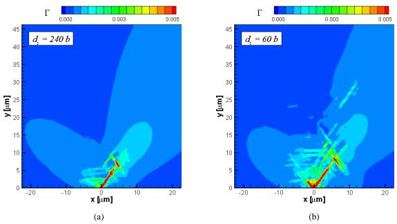
**Figure 10:** Contours of total slip  $\Gamma = \sum |\gamma^{(\alpha)}|$  around the crack tip at  $K_I/K_0 = 0.08$  for two cases with different slip plane spacing: (a)  $d_s = 240 \ b$ , (b)  $d_s = 60 \ b$ .
