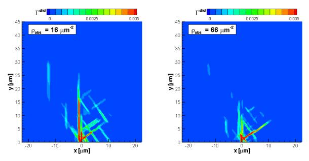
**Figure 16**: Contours of total slip  $\Gamma = \sum \left| \gamma^{(\alpha)} \right|$  (contributed only by the dislocations) around the crack tip at  $K_l/K_0 = 0.08$  for the bcc-like orientation and two different obstacle densities: (a)  $\rho_{obs} = 16 \mu m^{-2}$ , (b)  $\rho_{obs} = 66 \mu m^{-2}$ .
