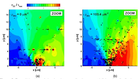
(a) (b) Figure 5: Zoom (15 x 15  $\mu$ m) showing the normalized stress and dislocation distribution at  $K_I/K_0 = 0.08$  for the two limiting cases: (a)  $\rho_{obs} = 0~\mu m^{-2}$ , (b)  $\rho_{obs} = 103.4~\mu m^{-2}$
