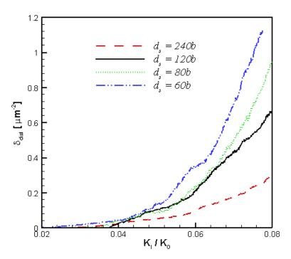
**Figure 12**: Dislocation density measured over the entire process windows versus the normalized applied stress intensity factor  $K_1/K_0$  for the different slip plane spacing for an FCC-like material.
