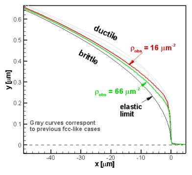
**Figure 17**: Crack shape at  $K_I/K_0 = 0.08$  for the bcc-like orientation and two different obstacle densities.
