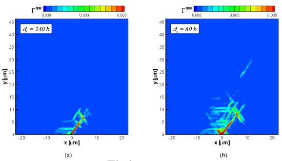
**Figure 11**: Contours of total slip  $\Gamma = \sum \left| \gamma^{(\alpha)} \right|$  (contributed only by the dislocations) around the crack tip at  $K_l/K_0 = 0$ . 08 for two cases with different slip plane spacing: (a)  $d_s = 240$  b, (b)  $d_s = 60$  b. Note the difference in the plastic zone  $(r_p)$  between the two cases.
