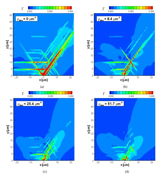
Figure 6: Contours of total slip  $\Gamma = \sum |\gamma^{(\alpha)}|$  around the crack tip at  $K_I/K_0 = 0.08$ . (a)  $\rho_{obs} = 0$  μm<sup>-2</sup>, (b)  $\rho_{obs} = 8.4$  μm<sup>-2</sup> (c)  $\rho_{obs} = 25.4$  μm<sup>-2</sup> (d)  $\rho_{obs} = 51.7$  μm<sup>-2</sup> (e)  $\rho_{obs} = 103.4$  μm<sup>-2</sup> (f) Elastic solution.
