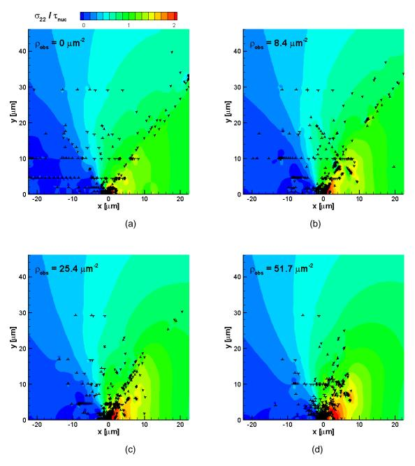
**Figure 4**: Normalized opening stress  $\sigma_{22}/\tau_{nuc}$  and dislocation distribution at  $K_l/K_0 = 0.08$ . (a)  $\rho_{obs} = 0$   $\mu m^{-2}$ , (b)  $\rho_{obs} = 8.4 \ \mu m^{-2}$  (c)  $\rho_{obs} = 25.4 \ \mu m^{-2}$  (d)  $\rho_{obs} = 51.7 \ \mu m^{-2}$  (e)  $\rho_{obs} = 103.4 \ \mu m^{-2}$  (f) Elastic solution.
