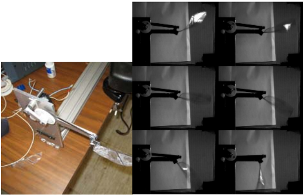
Fig 12. Wing tester and camera images of a test wing at 20Hz.
