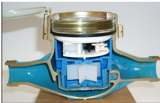
Household water meter
