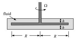
a. If the torque required to rotate the disk at  $\Omega = 900$  rpm is 0.537 N·m, determine the dynamic viscosity of the fluid. You may neglect the viscous forces acting on the rim of the disk and on the vertical shaft.
