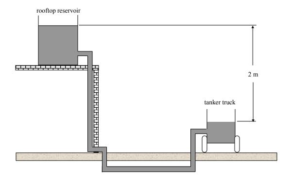
Water at 10 °C (kinematic viscosity of 1.307\*10<sup>-6</sup> m<sup>2</sup>/s) is to flow from a roof-top reservoir to a tanker truck through a cast iron pipe (roughness of 0.26 mm) of length 20 m at a flow rate of 0.0020 m<sup>3</sup>/s. The roof-top tank water level is located 2 m above the tanker truck fluid level. The system contains a sharp-edged entrance, six threaded 90° elbows, and a sharp-edged exit. Determine the required pipe diameter for the given flow conditions.
