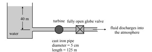
Determine the power, in W, extracted by the turbine in the system shown below. The pipe entrance is sharp-edged and the volumetric flow rate is  $0.004 \text{ m}^3$ /s. The density of water is 998 kg/m<sup>3</sup> and the kinematic viscosity is  $1.005e-6 \text{ m}^2$ /s.
