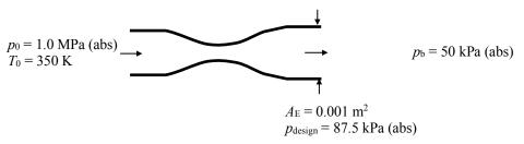
The exit Mach number may be found using the isentropic pressure ratio at the exit. Since the back pressure is less than the design pressure (underexpanded conditions), the exit pressure will be equal to the design pressure.
