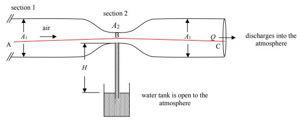
Apply Bernoulli's equation along a streamline from point B to point C in order to determine the pressure at point B. Neglect changes in elevation.
