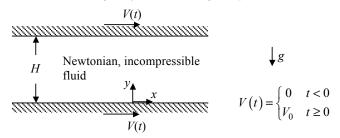
Assume at time t < 0 the entire system is at rest. For  $t \ge 0$ , the walls are impulsively started and move at a constant speed  $V_0$  in the +x-direction.
