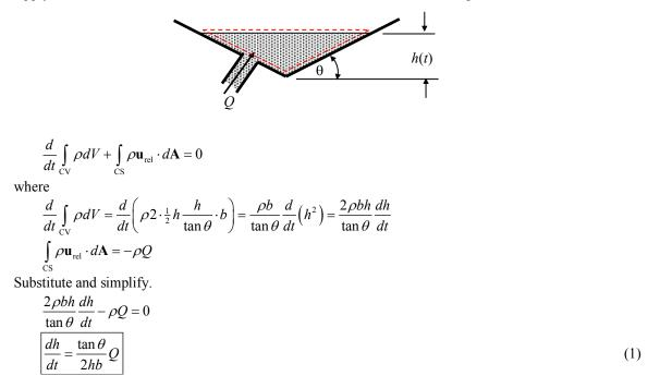
Solve the differential equation to determine the time required for a specified change in the liquid level.
