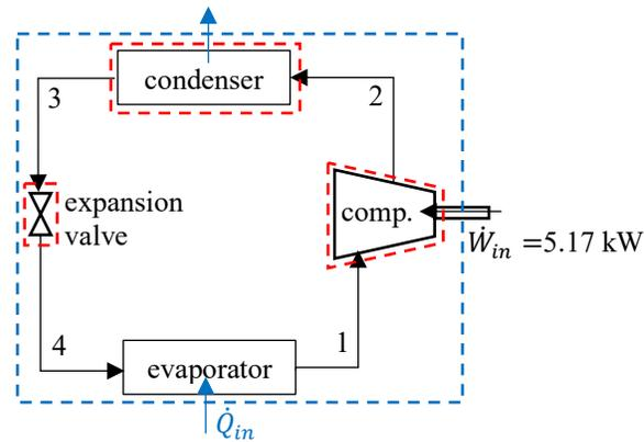
A heat pump's coefficient of performance, in terms of the variables used in the schematic (and using the blue CV shown), is,
