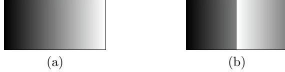
Figure 5: An illustration of why pixel-intensity variance is ill-suited as a measure of segment homogeneity. The intensity of image (a) varies uniformly from 0 at the left to 255 at the right. The intensity of image (b) varies uniformly from 0 at the left to 128 in the center, then abruptly changes to 255, and finally varies uniformly from 255 to 129 at the right. While these two images have the same statistical properties, image (a) appears to contain a single segment while image (b) appears to contain two segments.
