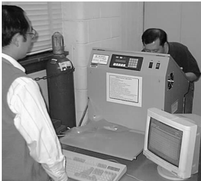
The olfactometer presents a precisely diluted odor sample to each panelist.
