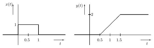
(a) (5 pts) Find the output of the system corresponding to the input x(0.5t), and sketch it on the graph provided on the next page.
