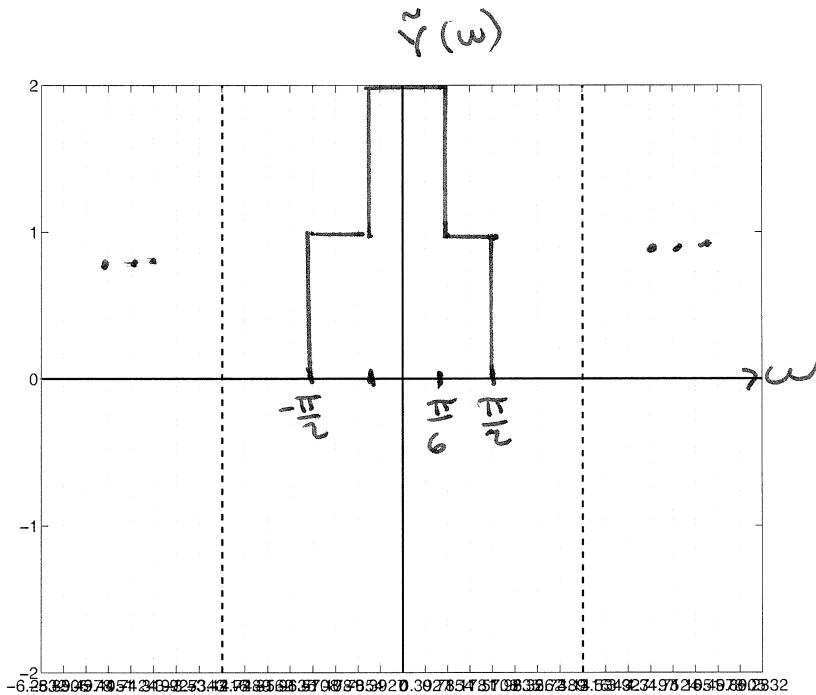
$$Y(\omega) = X(\omega - s) + X(\omega + s) \quad X(\omega) = \text{rect}\left(\frac{\omega}{2s}\right)$$
