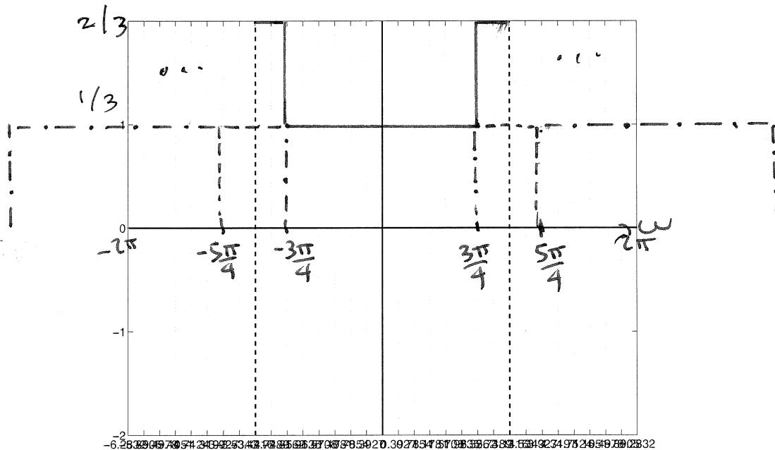
$x(3t) \xrightarrow{\text{FT}} \frac{1}{3} X\left(\frac{\omega}{3}\right)$  expansion by a factor of 3
