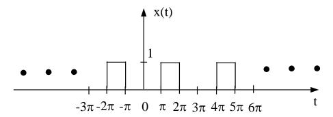
A discrete-time signal is created by sampling x(t) according to  $x[n] = x(nT_s)$  for  $T_s = \frac{3\pi}{8}$ .
