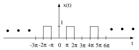
through the system  $y(t) = \int_{t-\pi}^{t+\pi} x(\tau) d\tau$ . NEXT, consider the CT signal  $x_4(t)$  defined in terms of y(t) as  $x_4(t) = y(t) * \left\{ \frac{\sin(2t)}{\pi t} \right\}$ , where \* denotes convolution. A DT signal is obtained by sampling  $x_4(t)$  according to  $x_4[n] = x_4(nT_s)$  for  $T_s = \frac{2\pi}{4}$ .
