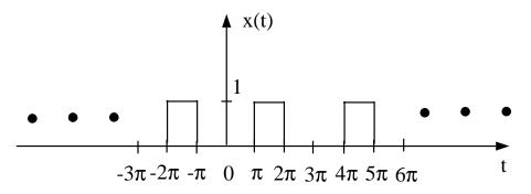
A discrete-time signal is created by sampling  $x_3(t)$  according to  $x_3[n] = x_3(nT_s)$  for  $T_s = \frac{2\pi}{4}$ .
