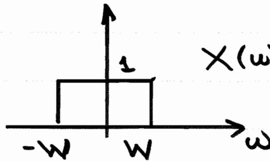
$$X(\omega) = \text{rect}\left(\frac{\omega}{2W}\right)$$
