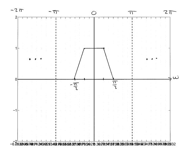
$$H(\omega) = -j H_{LP}(\omega - \frac{\pi}{2}) + j H_{LP}(\omega + \frac{\pi}{2})$$
