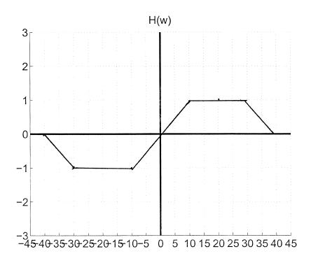
**Problem 2** (b). Determine the Fourier Transform of the signal x(t) below.
