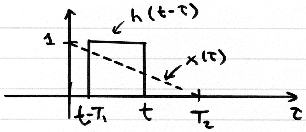
$$y(t) = \int_{t-T_1}^t \left(1 - \frac{\tau}{T_2}\right) d\tau = \left[ \tau - \frac{1}{2T_2} \tau^2 \right]_{t-T_1}^t$$
