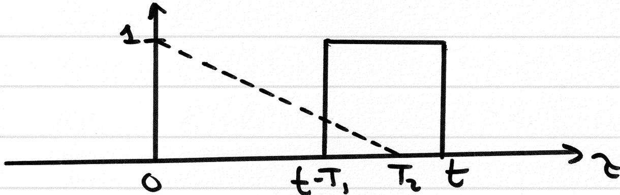
$$y(t) = \int_{t-T_1}^{T_2} \left(1 - \frac{\tau}{T_2}\right) d\tau = \left[\tau - \frac{1}{2T_2} \tau^2\right]_{t-T_1}^{T_2}$$
