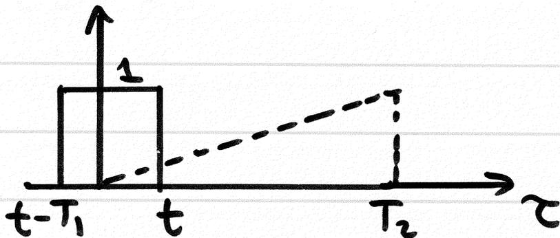
$$y(t) = \int_0^t \frac{\tau}{T_2} d\tau = \frac{1}{T_2} \left[ \frac{\tau^2}{2} \right]_0^t = \frac{t^2}{2T_2}$$
