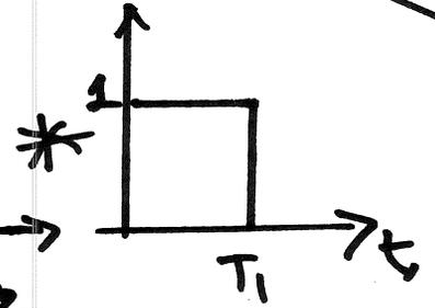
$$\underbrace{\{u(t) - u(t - T_1)\}}_{\text{rect}\left(\frac{t - \frac{T_1}{2}}{T_1}\right)} * \underbrace{\left\{- (t - T_2) (u(t) - u(t - T_2))\right\}}_{\text{rect}\left(\frac{t - \frac{T_2}{2}}{T_2}\right)} =$$
