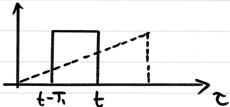
$$y(t) = \int_{t-T_1}^t \frac{t}{T_2} d\tau = \left. \frac{1}{2T_2} \tau^2 \right|_{t-T_1}^t$$
