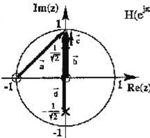
$$H(e^{j\pi/2}) = \underline{\vec{a}} + \underline{\vec{b}} - \underline{\vec{c}} - \underline{\vec{d}}$$
