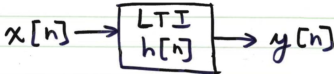
$$r_{yx}[\ell] = r_{xx}[\ell] * h[\ell] \quad \left. \begin{array}{l} \text{cross-} \\ \text{correlation} \\ \text{between input} \\ \text{and output} \end{array} \right\}$$
