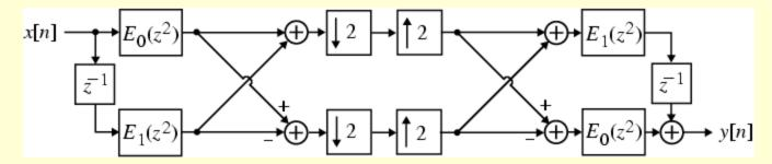
• Making use of the cascade equivalences, the above structure can be further simplified as shown below
