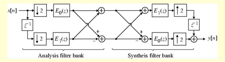
• Substituting the polyphase representations of the analysis filters we arrive at the expression for the distortion function T(z) in terms of the polyphase components as
