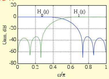
• The program then computes the amplitude distortion  $|H_0(e^{j\omega})|^2 + |H_1(e^{j\omega})|^2$  in dB as shown below
