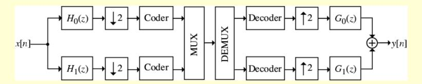
• The analysis filters  $H_0(z)$  and  $H_1(z)$  have typically a lowpass and highpass frequency responses, respectively, with a cutoff at p/2
