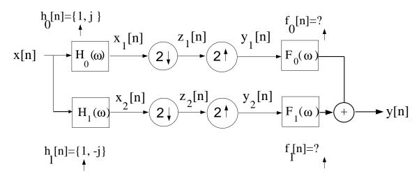
where  $z_i[n] = x_i[2n]$ , i = 1, 2 and  $y_i[n] = \sum_{\ell=-\infty}^{\infty} z_i[\ell] \delta[n-2\ell]$ , i = 1, 2. Determine the numerical values of  $f_0[n]$ , n = 0, 1 and  $f_1[n]$ , n = 0, 1, such that y[n] = 2x[n-1] for any input sequence x[n].
