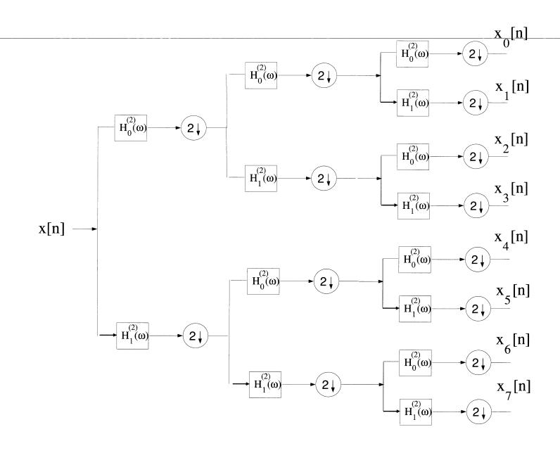
**Problem 2.** In Matlab Homework 2, you used Noble's Identities to convert the Tree-Structured subbander on the previous page to the regular maximally decimated subbander, obtaining products of the form:
