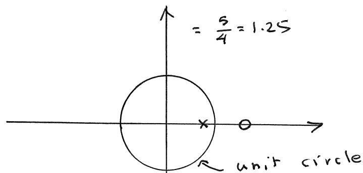
$$H_1(\omega) = \frac{-1 + P_1 e^{j\omega}}{e^{j\omega} - P_1} = -e^{j\omega} \frac{(-e^{-j\omega} - P_1)}{e^{j\omega} - P_1}$$
