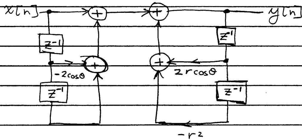
$$\begin{aligned} y[n] = & 2r \cos \theta y[n-1] - r^2 y[n-2] \\ & + x[n] - 2 \cos \theta x[n-1] + x[n-2] \end{aligned}$$
