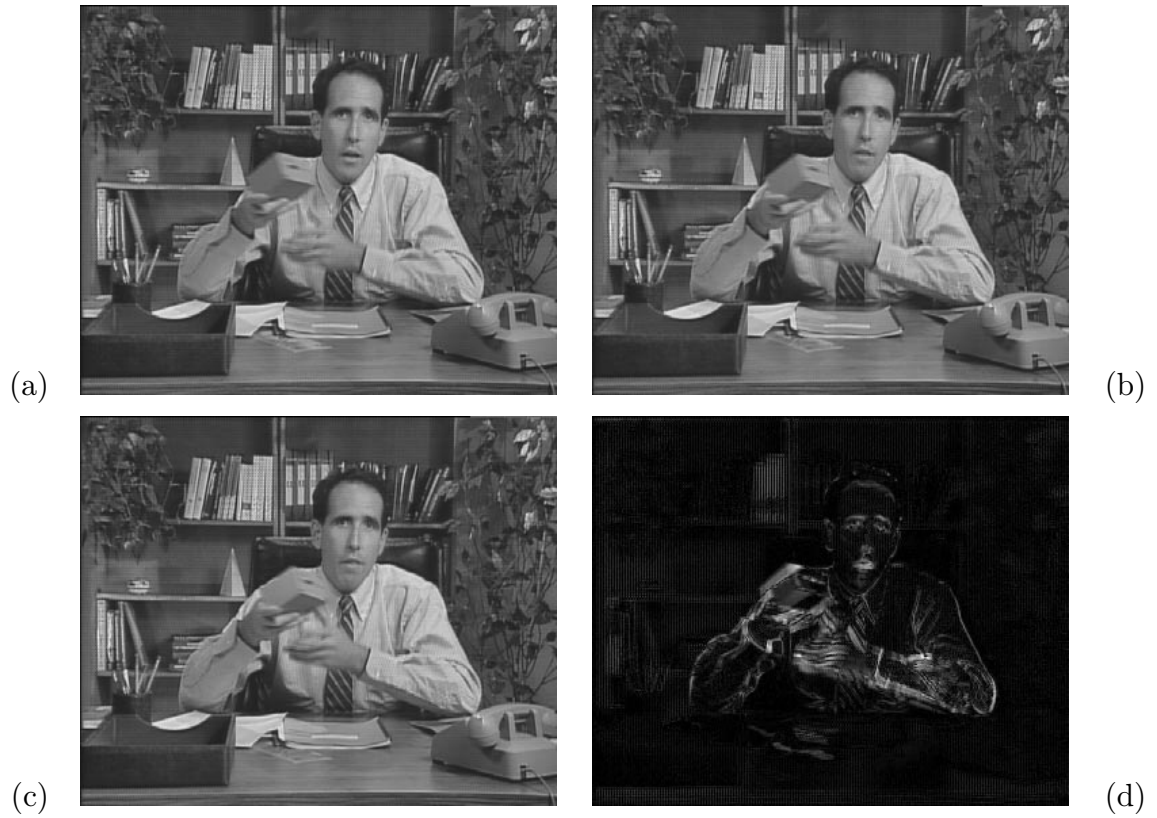
Fig. 4.14. Frames (a) 13, (b) 14, and (c) 15 of the salesman sequence. (d) Shows the average absolute difference between frames 13 and 14 and frames 14 and 15.
