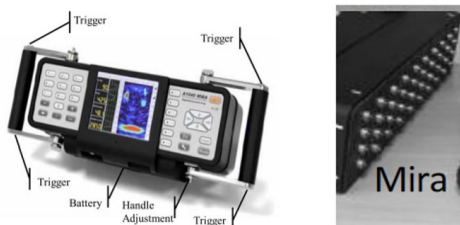
Fig. 15. A picture of the MIRA device used for the experimental data. The device has 10 columns of transducers, where each column acts as a single transducer.
