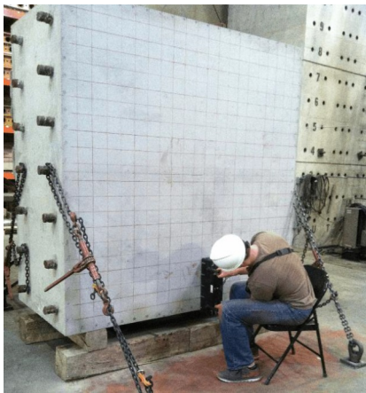
Fig. 10. The concrete specimen used for the experimental data [33]. 20 defects are embedded in the specimen.
