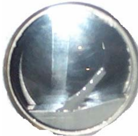
Figure 19: 15° Ramp Oil Flow Shock Visualization
