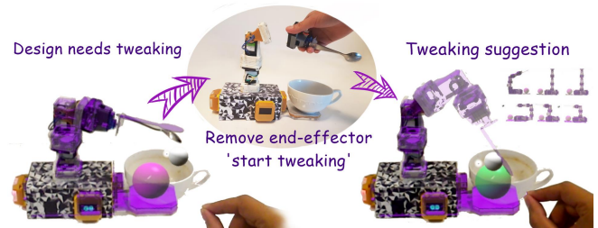
Figure 8. Tweaking with MRI: virtual tryout for functional improvement. Tweaking a robot manipulator setup so that the spoon tip can reach inside the bowl.
