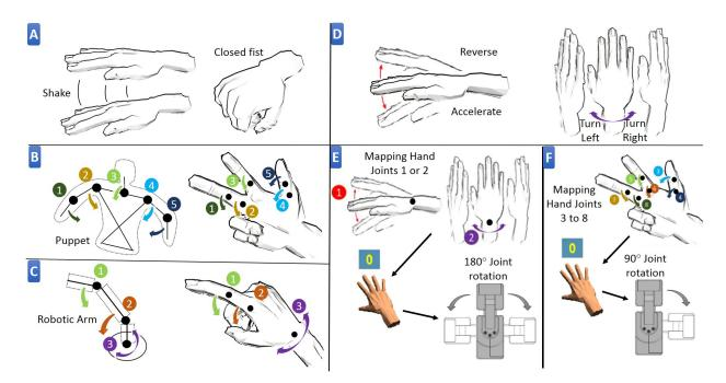
Figure 7. Interaction methods: (a) Global Gestures; Gestures for (b) Puppet Shaped Constructions (c) Robotic Arm shaped constructions (d) Vehicular constructions; User Defined gesture mapping for custom robots (e) Hand joints 1 or 2 (f) Hand joints 3 to 8
