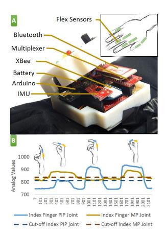
Figure 4. (a) Electronics in the Glove-based Controller (b) Analog readings of the flex sensor at Index finger PIP joint and MP joint for different finger orientations
