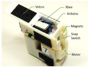
Figure 5. Electronics in the Joint Modules
