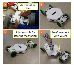
Figure 11. Learning by prototyping (a) Inserting anti-rotation bar to the two wheeled car (b) 4 wheeled car (c) 4 wheeled car with steering mechanism (d) Final 4 wheeled car with robotic arm
