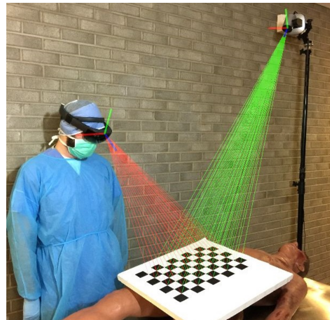
Figure 3: Calibration process. The overhead camera (green ray visualization) is registered with respect to the camera built into the AR HMD (red rays) using a calibration checkerboard.
