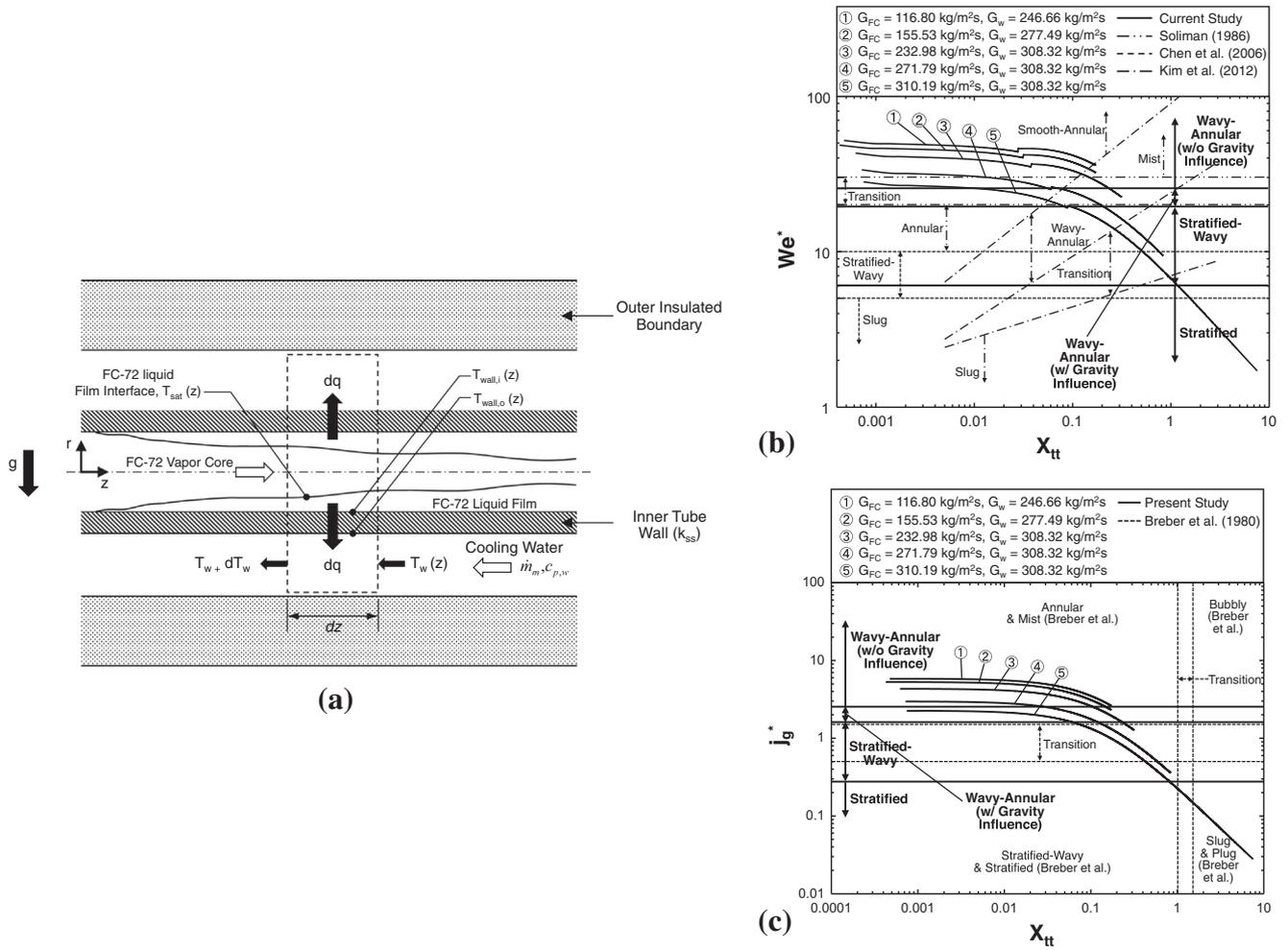
**Fig. 4.** (a) Thermal model used to determine the local condensation heat transfer coefficient for FC-72. (b) Operating conditions for heat transfer module superimposed on prior flow regime maps based on  $We^*$  versus  $X_{tt}$ , along with predictions of Soliman [24], Chen et al. [25] and Kim et al. [20]. (c) Operating conditions for heat transfer module superimposed on prior flow regime map based on  $J_g^*$  versus  $X_{tt}$ , along with predictions of Breber et al. [22].
