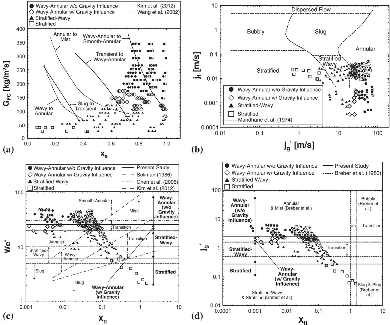
**Fig. 3.** Comparison of present flow regime data with flow regime maps of: (a) Wang et al. [29] and Kim et al. [20], (b) Mandhane et al. [21], (c) Soliman [24], Chen et al. [25] and Kim et al. [26], and (d) Breber et al. [22].
