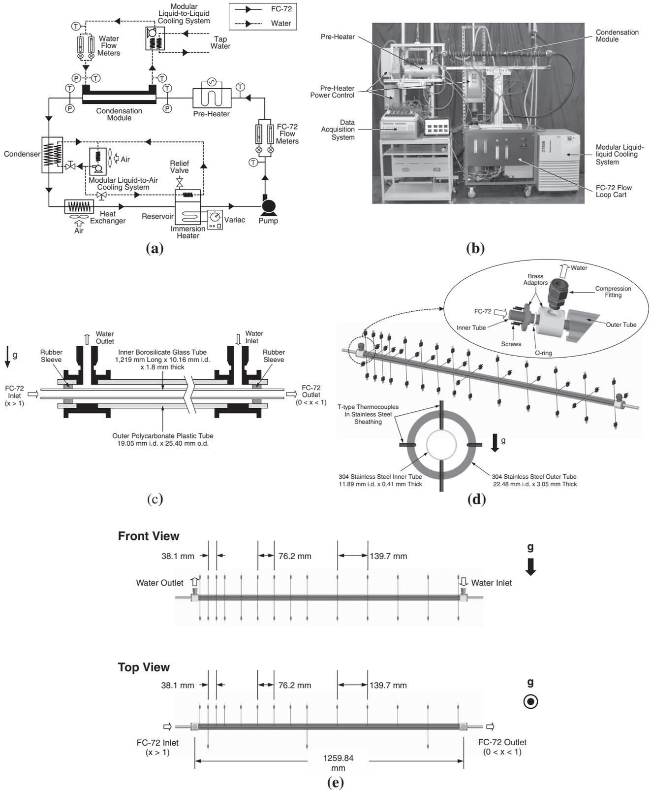
**Fig. 1.** (a) Schematic diagram of condensation facility. (b) Photo of facility. (c) Construction of flow visualization module. (d) Construction of heat transfer module. (e) Location of thermocouples for temperature measurements of outer wall of inner tube and cooling water in heat transfer module.
