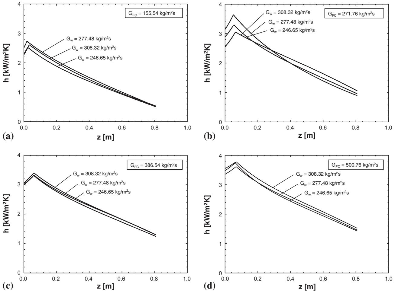
Fig. 7. Axial variation of experimentally determined condensation heat transfer coefficient in heat transfer module for different water mass velocities and FC-72 mass velocities of (a)  $G_{FC} = 155.54 \text{ kg/m}^2 \text{ s}$ , (b)  $G_{FC} = 271.76 \text{ kg/m}^2 \text{ s}$ , (c)  $G_{FC} = 386.54 \text{ kg/m}^2 \text{ s}$ , and (d)  $G_{FC} = 500.76 \text{ kg/m}^2 \text{ s}$ .
