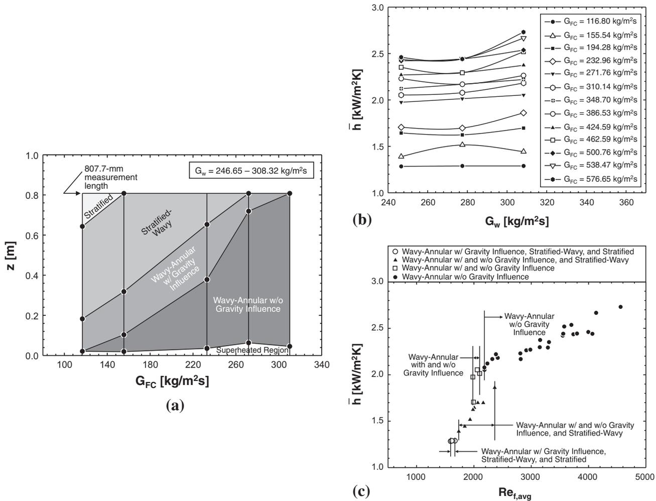
**Fig. 9.** (a) Variations of flow regimes along condensation length for different FC-72 mass velocities. (b) Variation of experimentally-determined average condensation heat transfer coefficient with water mass velocity for different FC-72 mass velocities. (c) Variation of experimentally-determined average condensation heat transfer coefficient with film Reynolds number averaged over two-phase region.
