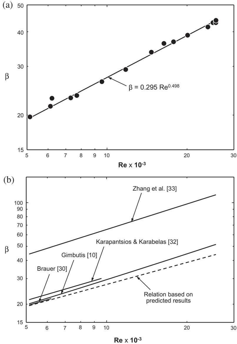
Fig. 8. (a) Curve fit to predicted film thickness for  $Re = 5130\text{--}25,680$  and  $Pr = 2.55\text{--}6.87$ . (b) Comparison of present film thickness relation with prior correlations.
