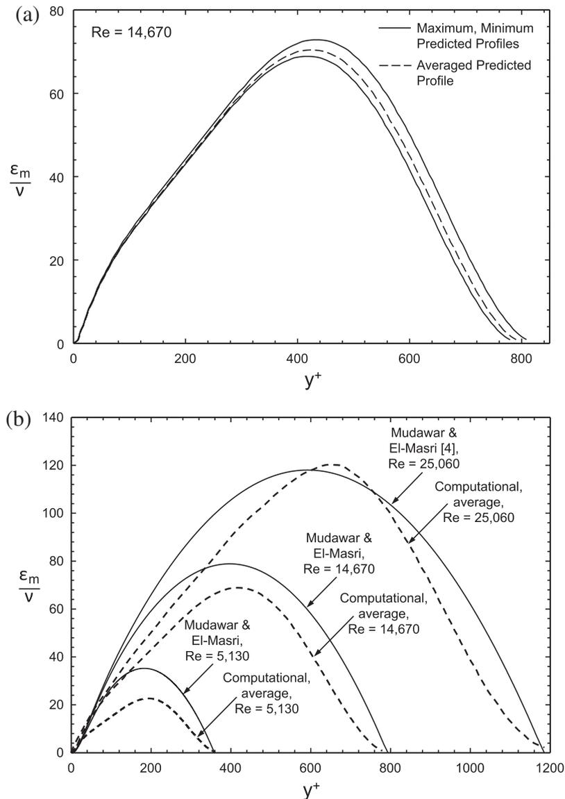
Fig. 11. (a) Maximum, minimum and average predicted eddy diffusivity profiles for  $Re = 14,670$ . (b) Comparison of predicted eddy diffusivity profile with Mudawar and El-Masri's [4] for  $Re = 5,130, 14,670$  and  $25,060$ .
