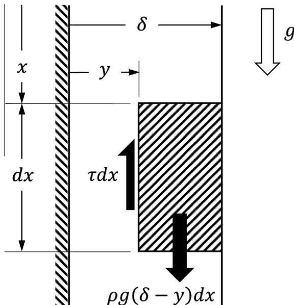
Fig. 1. Force balance for control volume of fully developed free-falling film.
