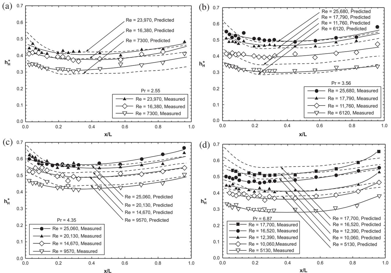
Fig. 9. Variations of measured and predicted dimensionless heat transfer coefficient along heated length of test section for (a)  $Pr = 2.55$ , (b)  $Pr = 3.56$ , (c)  $Pr = 4.35$ , and (d)  $Pr = 6.87$ .
