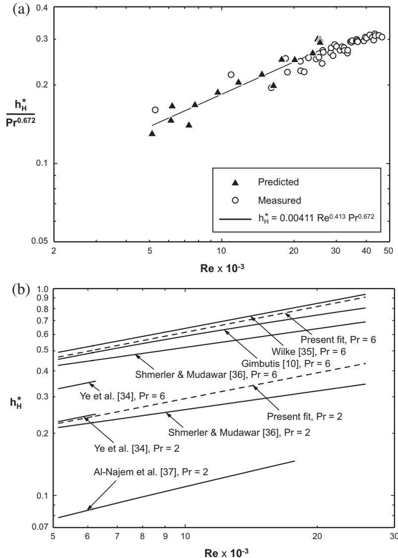
Fig. 10. (a) Comparison of measured and predicted heat transfer coefficient for  $Re = 5130–25,680$  and  $Pr = 2.55–6.87$ . (b) Comparison of present heat transfer relation with prior correlations.
