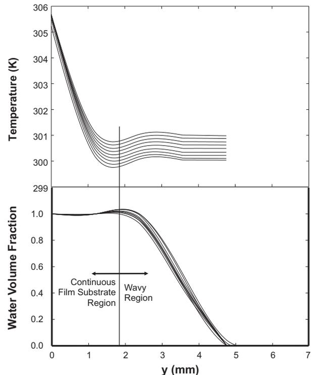
Fig. 7. Variations of film temperature profile at different subintervals within the period of a single dominant wave, and corresponding water volume fraction profiles for  $x = 390.5$  mm,  $Re = 25,060$ ,  $Pr = 4.35$  and  $q''_w = 55,000$  W/m<sup>2</sup>.
