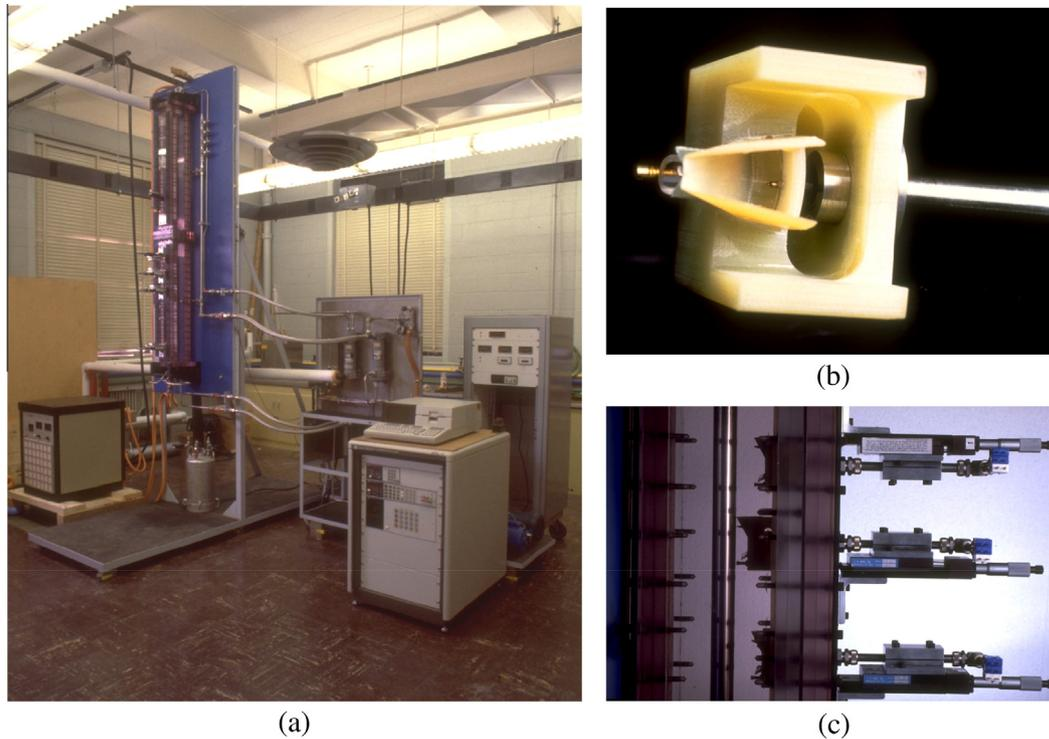
Fig. 3. Photos of (a) falling film facility, (b) top view of sampling scoop, and (c) stainless steel tube and sampling scoops mounted on micrometer stages.
