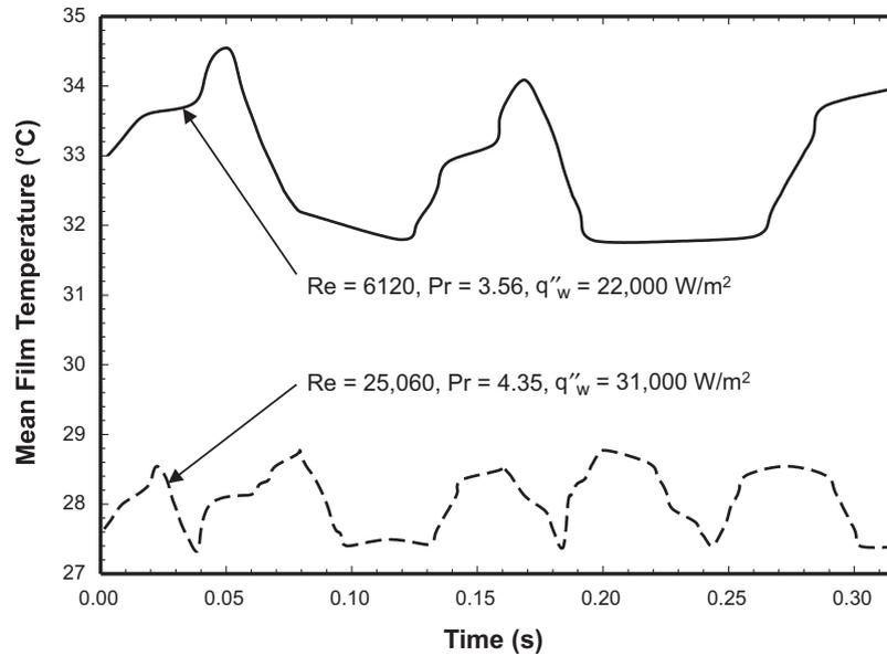
Fig. 6. Predicted temporal records of mean film temperature at  $x = 350$  mm for two cases.
