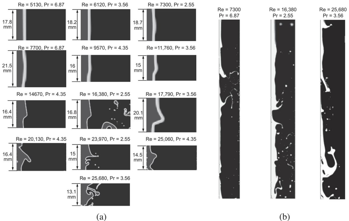
**Fig. 5.** (a) Dominant repeated wave shape for 13 test cases. (b) Variations of interfacial shape for 3 test cases.
