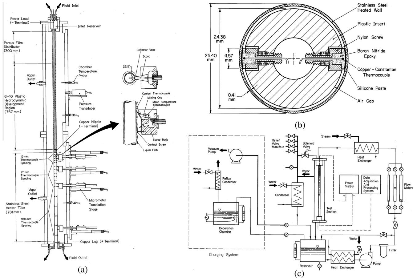
**Fig. 2.** (a) Cut-away view of test chamber. (b) Cross-sectional view of inner thermocouples. (c) Schematic diagram of flow loop.
