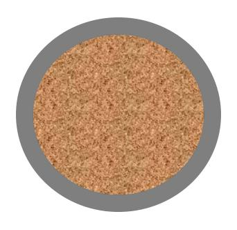
RAP aggregate with oxidized binder film
