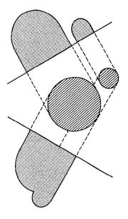
**Fig. 1.1:** Two projections are shown of an object consisting of a pair of cylinders.
