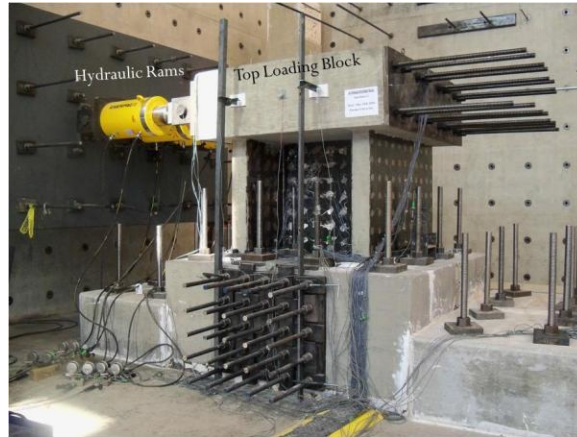
Figure 4 Photograph of In-Plane Specimen and Setup
