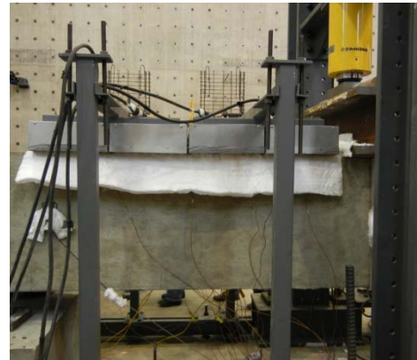
Fig. 4: Heater Test Setup over Shear Span
