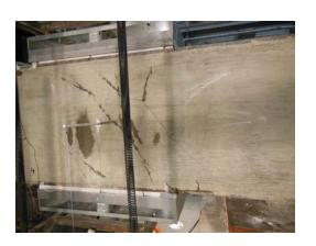
Figure 9 - Diagonal Shear Crack Occurrence of in the heating phase
