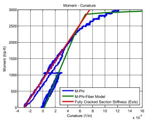
Figure 7 - Moment-curvature behavior of Specimen T1, zoom into initial loading stage
