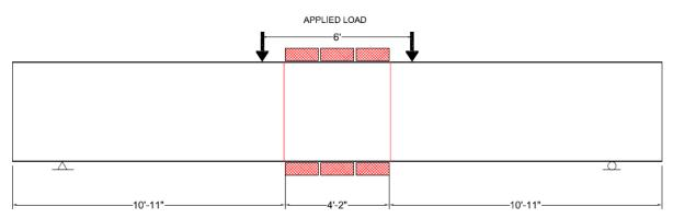
Figure 2 - Elevation View with Heaters of Specimen T1
