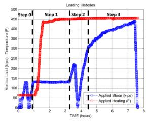
Figure 3 - Applied Load and Steel Plate Temperature Histories of Specimen T1
