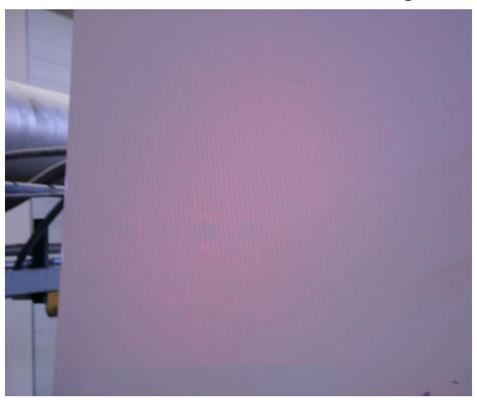
Particles traverse fringes in flow, scatter light at a frequency proportional to their axial speed.
