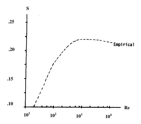
Figure 12-2. Sketch of Strouhal Number vs. Reynolds Number for a Cylinder
