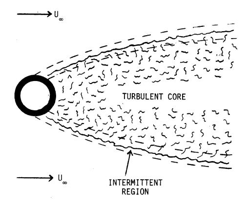
Figure 4. Schematic of a Wake Shadowgraph
