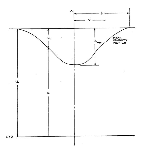
Figure 5. Velocity Profile in a Wake
