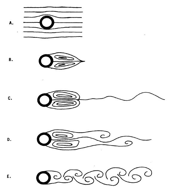
Figure 1. Flow Patterns in the Wake of a Circular Cylinder. Flow is from Left to Right.
