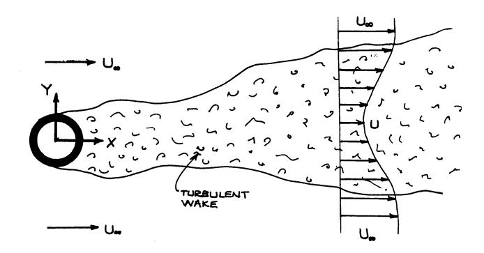
Figure 3. Sketch of a Turbulent Wake, in a Lab-Fixed Frame
