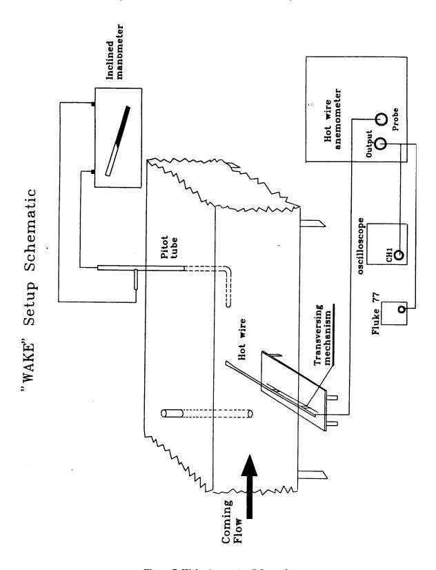
Figure 7 Wake Apparatus Schematic
