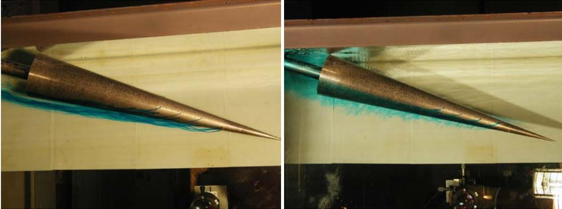
**Figure 5** Flow visualization for  $18.25^\circ$  angle of attack. Left is with freestream velocity 3.0 in/sec and shows a laminar boundary layer. Right is for freestream velocity 10.5 in/sec and shows a turbulent boundary layer.
