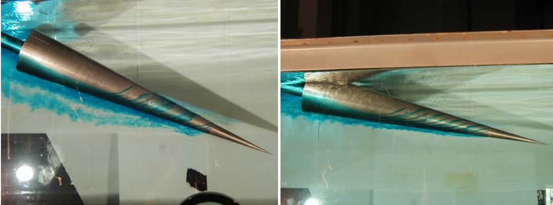
**Figure 7 Left is a visualization for  $25.5^\circ$  angle of attack and freestream velocity 10.5 in/sec. This is a good view of turbulent boundary layer separation. Right is at  $14.5^\circ$  and freestream velocity 10.5 in/sec. This shows an attached, transitioning boundary layer.**
