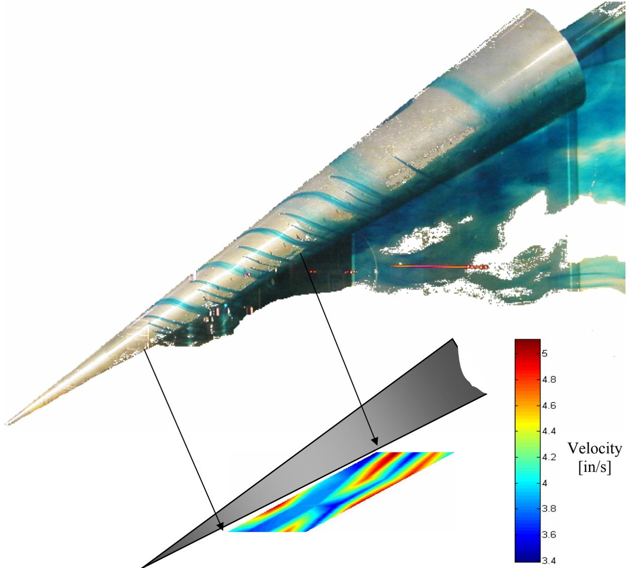
**Figure 11. Velocity profile in the wake of a cone with a freestream velocity of 4.7 in/s. Visualization of the flow behind the cone is provided for comparison.**
