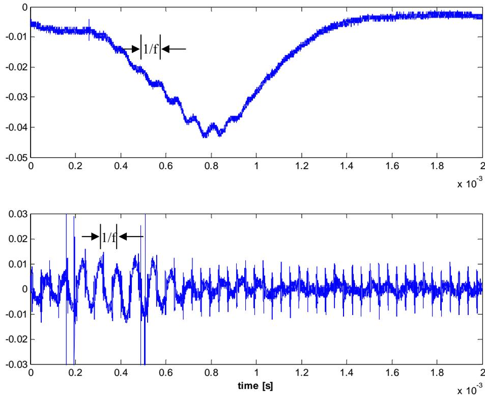
**Figure 8. Oscilloscope capture of a Doppler burst for a particle in a flow of 3 in/s (meter speed). Top shows raw data while bottom shows high-pass filtered data.**
