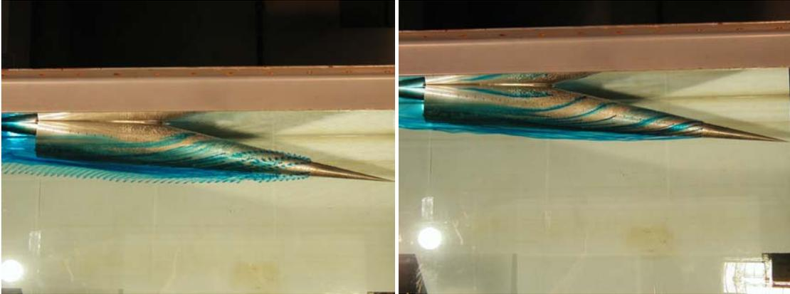
**Figure 3** Flow visualization for  $10.0^\circ$  angle of attack and freestream velocity 3.0 in/sec. The left picture shows flow with dye jets. Right shows normal dye flow.
