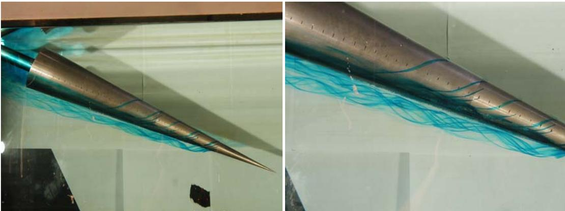
**Figure 4** Flow visualization for  $25.5^\circ$  angle of attack and freestream velocity 3.0 in/sec. The attached laminar boundary layer can be seen. Left shows the whole cone. Right is a close-up.
