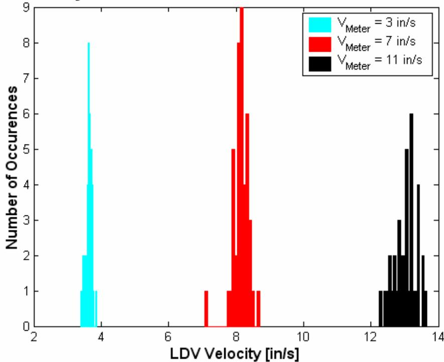
**Figure 10.** Flow speed distributions for LDV measurements in the Purdue water tunnel. The distributions widen as flow speed increases indicating that LDV measurements are most precise at low speeds.
