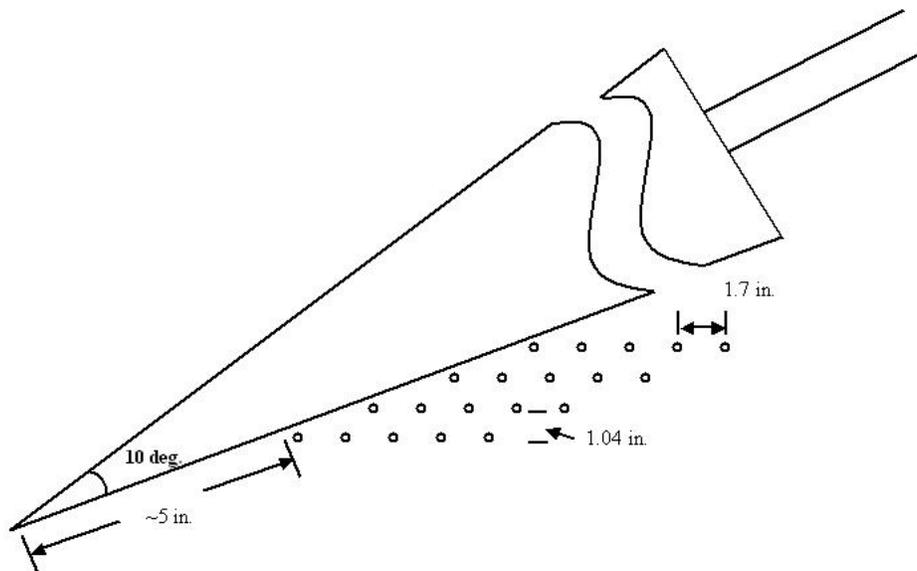
**Figure 2: Wake locations measured by LDV.**
