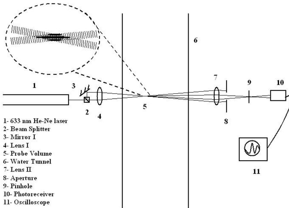
Figure 1 Diagram of LDV setup
