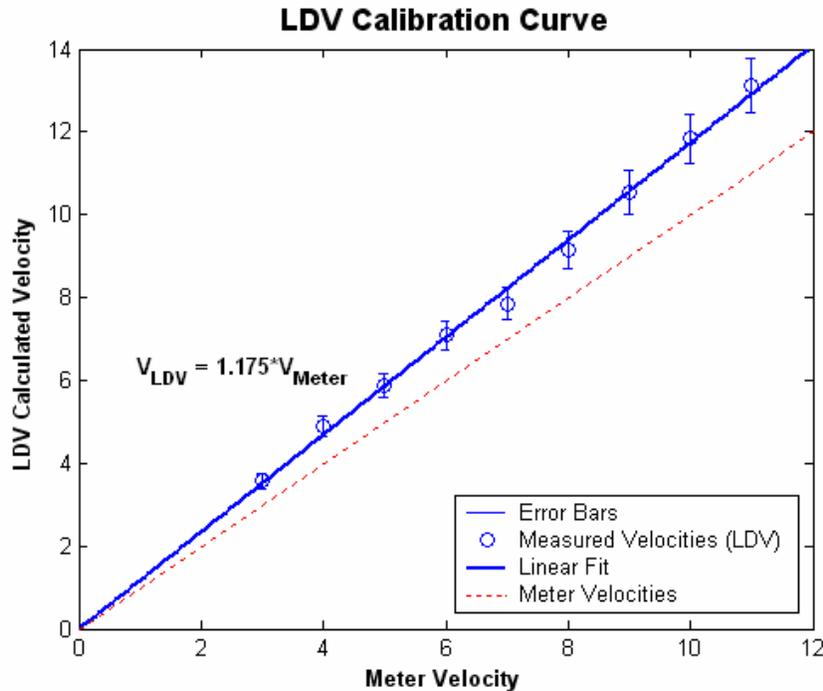
Figure 9. Velocity "calibration" curve comparing the flow velocity calculated through LDV with that read from a digital meter. Error bars representing 5% of the measured values are included and a linear fit is given. Also, the dotted line shows the expected 5% values for a perfectly calibrated flow meter.
