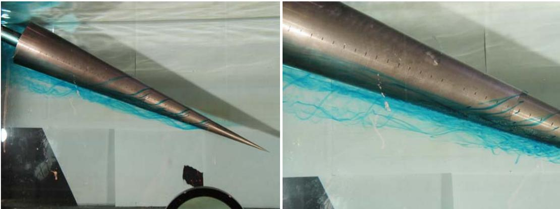
**Figure 6** Flow visualization for  $25.5^\circ$  angle of attack and freestream velocity 5.5 in/sec. Separation of the turbulent boundary layer can be seen. Left shows the whole cone. Right is a close-up.
