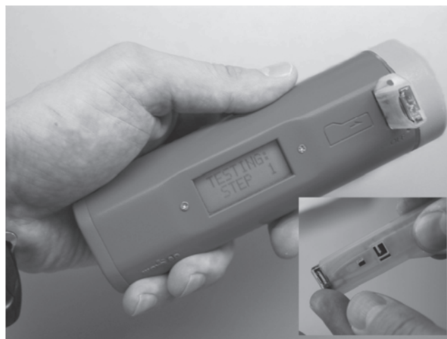
Figure 2: Highly portable, fully automated system for determining the composition of body fluids.
