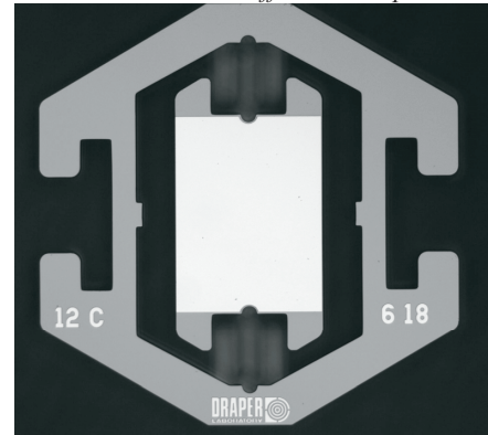
Figure 6. MEMS mirror photograph showing Au mirror and side notches (left and right side) for holding axles.
