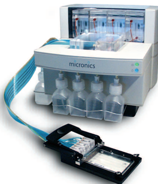
Figure 6. DEC Instrument and disposable interface—current prototype (shown without thermocycler attachment).
