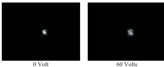
Figure 9. Images of a laser beam passing through the microlens with 0 V and 60 V applied.
