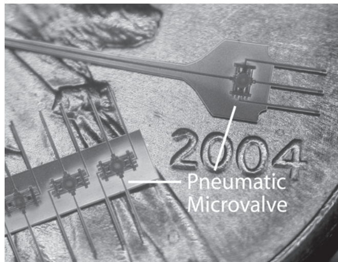
Figure 1. A drug delivery probe with integrated microvalves
