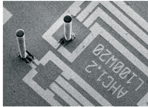
Figure 11. A pair of AHC sensors oriented orthogonally for resolving angular flow information.
