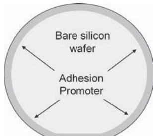
Fig. 5. Pattern of adhesion-promoter application
