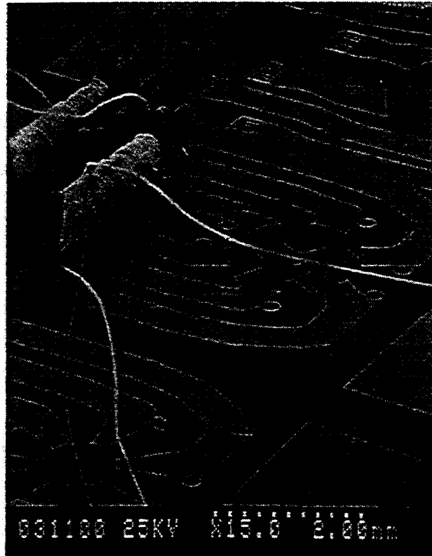
Figure 7: Peg assembly to increase structure height of a variable reluctance motor. Each layer is 250 \mu\text{m} thick.
