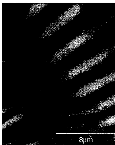
Figure 10: Imaged 8 \mu\text{m} wide disk drive track.
