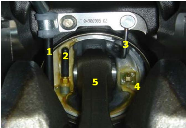
Fig. 2: Backside view of the prepared piston from the bottom of the oil pan. 1: transceiver antenna fixed to the oil cooling injector, a non moving part of the crankcase; 2: mounted sensor antenna inside on the bottom of the piston; 3: oil injector nozzle; 4: mounted SAW temperature sensor type TSEAS10 by SENSEOR; 5: Crankshaft.
