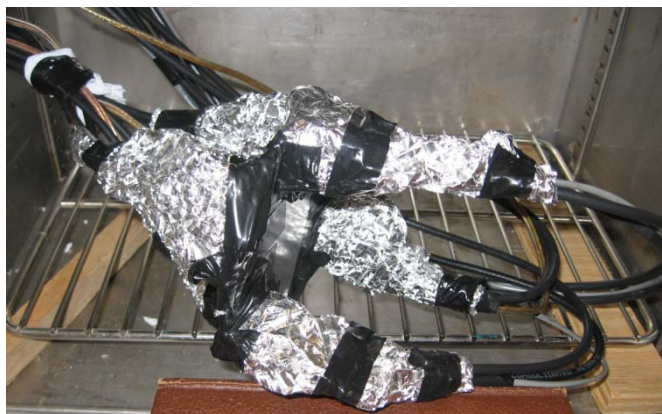
Figure 1. 6 Member Dual-Mode Oscillator Ensemble in Thermal Chamber with Aluminum Plate for Thermal Substrate and RF Shielding for Isolation.
