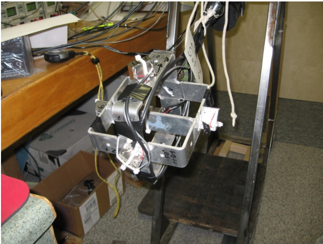
Figure 9. Cube/Pendulum Test Fixture for EQUATE Inertial Experiments.
