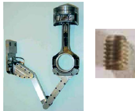
Fig. 1: Examples of piston temperature measurement approaches. Leftside : mechanical arm with joints. Rightside : metallurgical temperature sensor.
