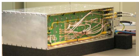
Figure 7. MWL Ground Terminal under assembly (top: steering unit with antenna and electronics unit, middle, bottom: electronics unit front panel, backplane).
