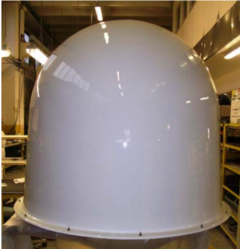
Figure 8. MWL Ground Terminal protective radome
