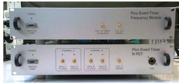
Figure 4. Two identical timing devices together with a power supply unit are placed in a 19" case and create a two-channel NPET timing device. The other 19" case includes the frequency multiplier 10 MHz to 200 MHz.
