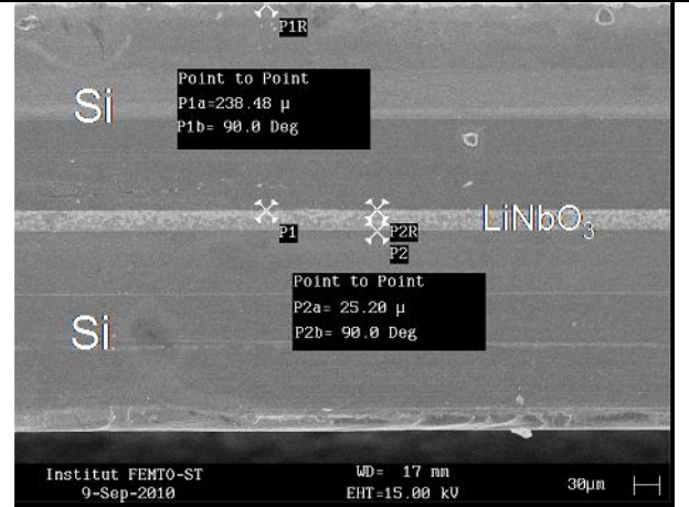
Fig.11. SEM view of a Si/thinned PPT/Si transducer
