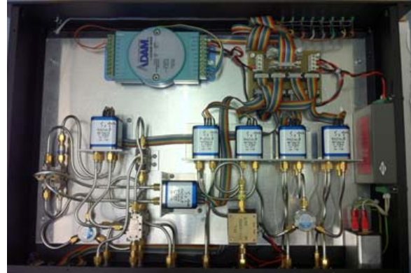
Figure 9 Final prototype of the new satellite simulator switch box designed and assembled at VSL.
