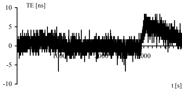
Figure 15. Time error obtained for synchronized oscillator measurement
