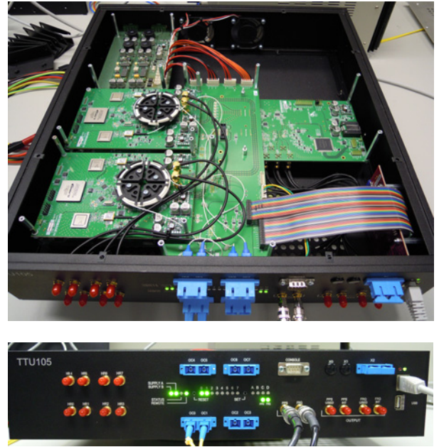
Figure 2. New, recently developed 2U (90 mm) hardware. Front panel and top view (without cover).
