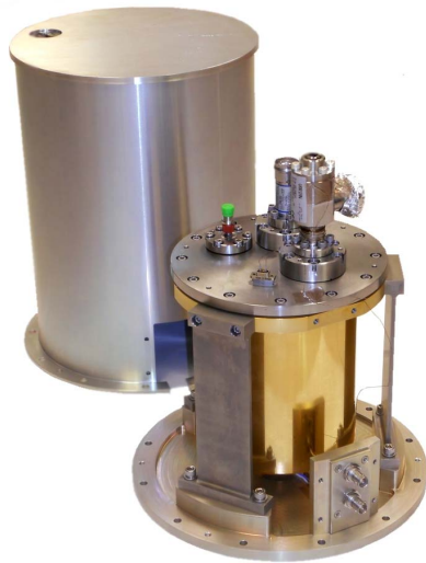
Figure 2. Reference cavity assembly with outer thermal shield removed
