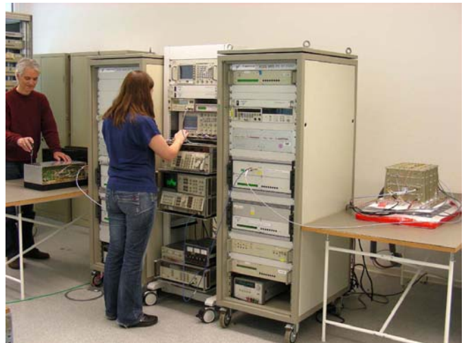
Figure 10. MWL end-to-end test set-up (MWL FS on the right, MWL GT electronics on the left, RF EGSE in the two center racks)
