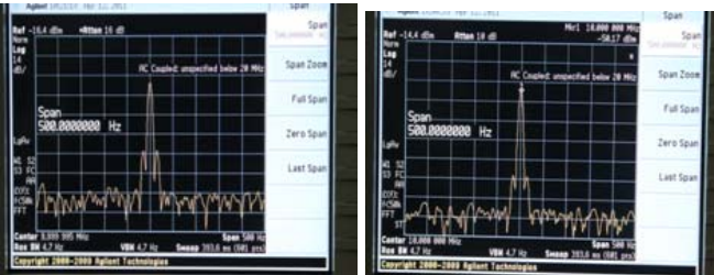
(c) Vibration without compensation G_{max}=4g, f=15Hz (d) Vibration with compensation k_p=4 G_{max}=4g, f=15Hz
