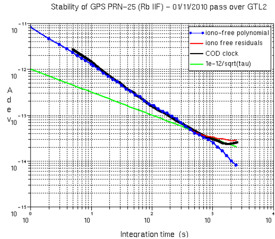
Figure 6. Stability of GPS PRN-25 Rb IIF using both methods on the iono-free combination
