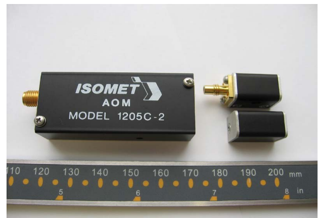
Fig. 1. Photographs of the "ISOMET" 1205-C2 AOM and couple of the "VNIIFTRI" AOM - RN.
