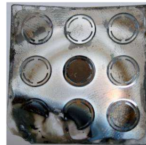
Fig. 1: DRIE of a small quartz wafer (1.5 x 1.5'' square)
