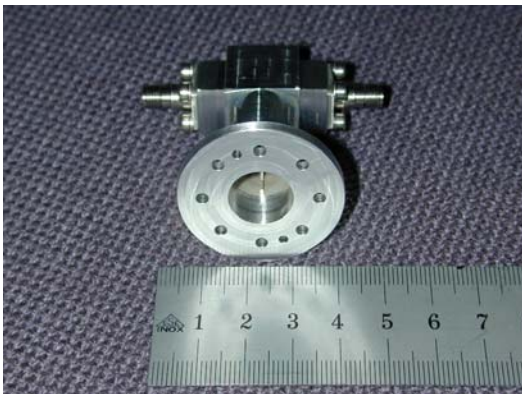
Figure 6. Engineering Model of the MWL Flight Segment Ku-Band antenna.
