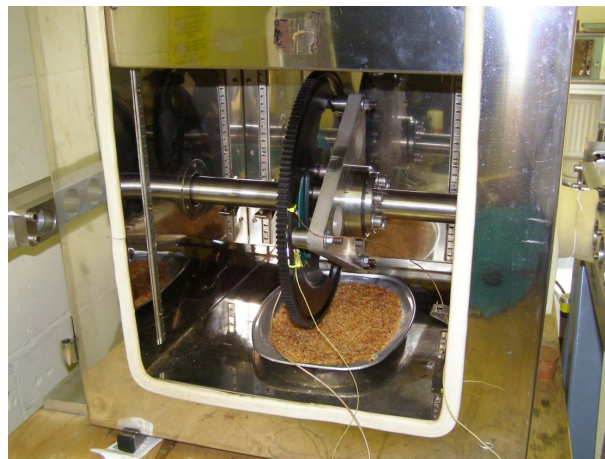
Figure 1. Calibration rig for the SAW flexplate torque transducer
