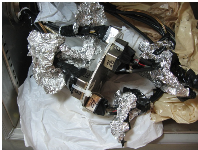
Figure 2. Detail showing oscillator packages, aluminum foil used to provide shielding and plastic used to improve thermal uniformity & reduce transients.
