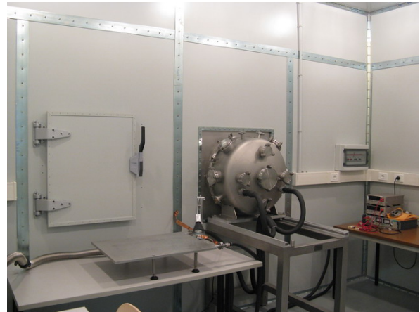
Figure 5. Thermal Vacuum chamber
