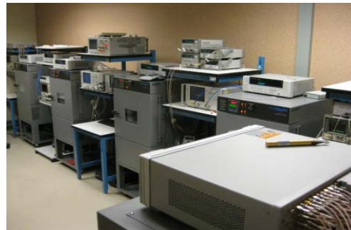
Figure 5. MEMS lab for the long term aging tests of pMEMS™ resonators and oscillators at Integrated Device Technology, Inc.
