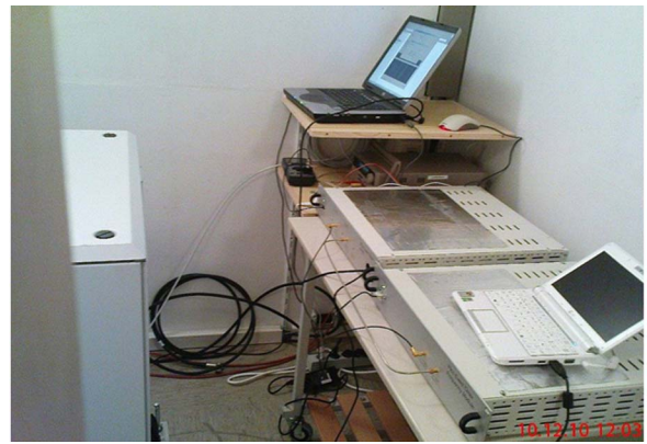
Figure 8. The experimental setup. There are from left to right the hydrogen maser EFOS SN 60, the data acquisition PC #1, the NPET timing device (channels #1 and #2), the frequency multiplier #1, and the data acquisition PC#2. The other maser EFOS SN 39 and frequency multiplier #2 were located in the next room.
