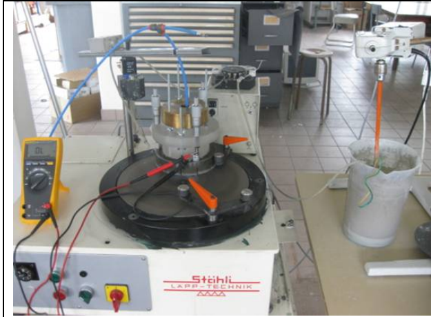
Fig.10. Photograph of the equipment used for lapping/polishing operations
