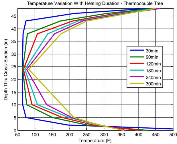
Figure 5 - Thru-depth temperature distributions obtained using the thermocouples on the thermocouple tree
