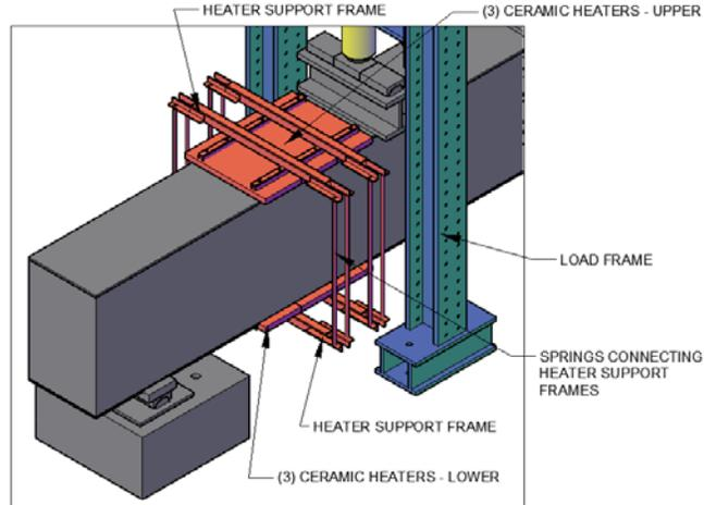
Figure 1 - Out-of-plane Shear + Thermal Loading Test Schematic Sketch
