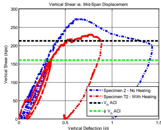
Figure 11 - Average load vs. average net mid-span deflection comparison of Specimen T2
